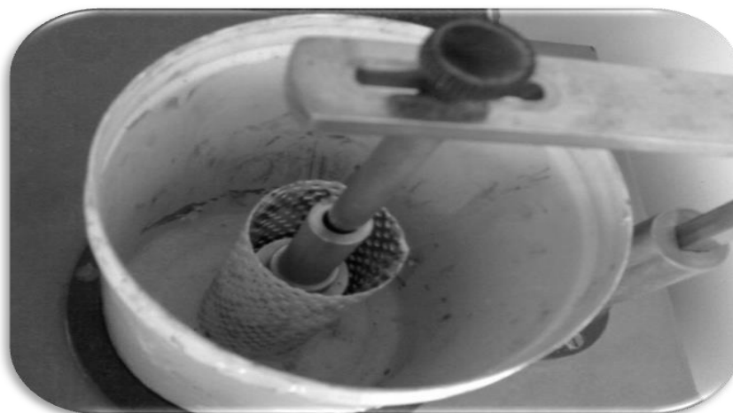
Figure No.1: Complete assembly of modified dissolution apparatus (Top View)
