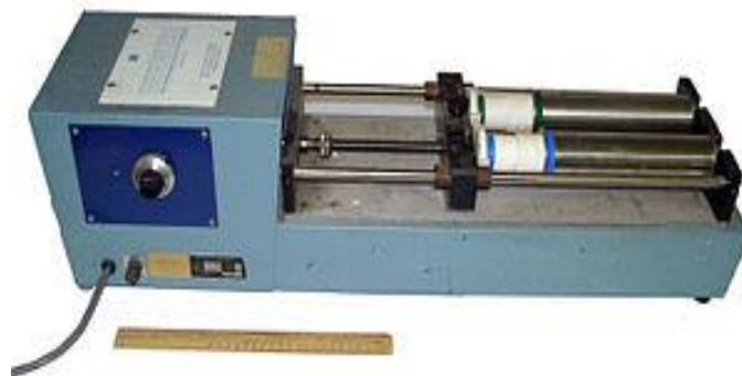
Figure. 7: An early, large model of insulin pump, 78 x 12 x 22 cm. 21
